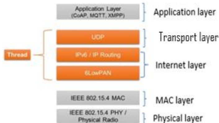
Fig.4. Thread protocol stack
